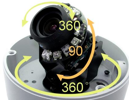
Adjust the focal and focus by sliding the sticks at the side of the lens.
