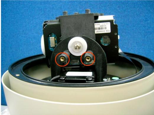
1. The positions marked with circles show the fixing holes of acrylic shield, i.e. four M3 screw holes.
